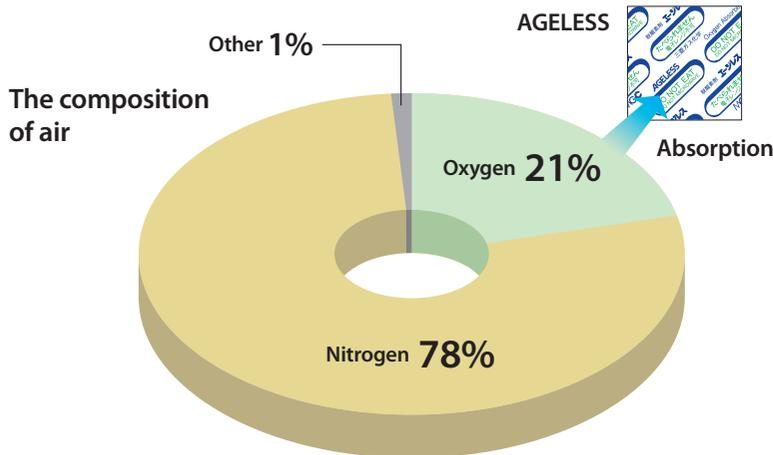
Oxygen makes up approximately 21% of the air in the atmosphere, however AGELESS absorbs all oxygen within a sealed container to create an oxygen free condition (maintaining an oxygen concentration of 0.1% or less). As AGELESS absorbs more oxygen, the volume decreases and the gas remaining within the sealed container becomes mostly nitrogen, an inert gas.
