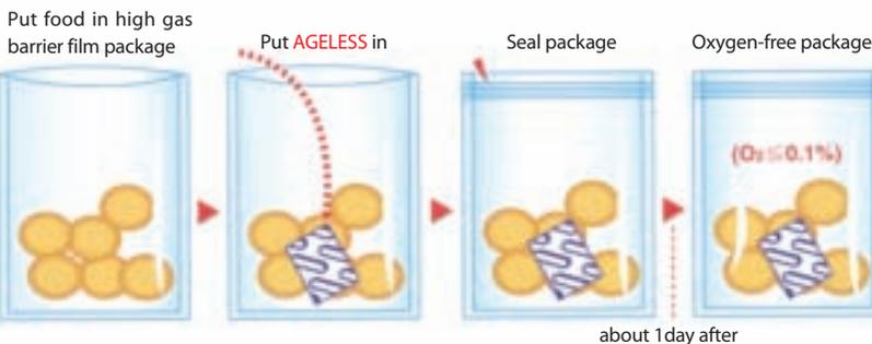
Conventional preservatives, antioxidants, gas flushing and vacuum packing often are not effective because they do not completely eliminate oxygen. Unique AGELESS oxygen absorber works to chemically absorb oxygen without altering product composition or purity without adding any chemicals or additives.
