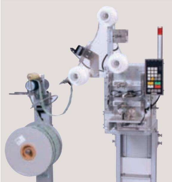
When connected to an automatic packing machine, pieces of AGELESS are cut from a roll and inserted one at a time. Its compact design means it can be installed and connected to existing packing machines.
