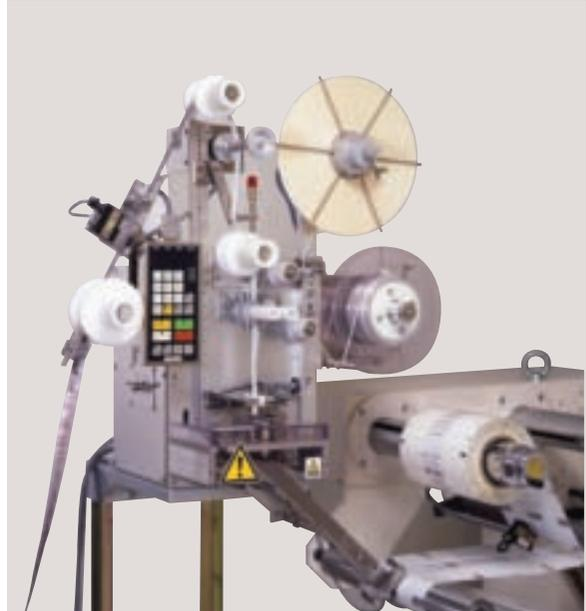
The machine affixes double-coated adhesive tape to AGELESS both packed in continuous rolls. The machine cuts the AGELESS and tape one by one in linkage with a packaging machine and fixes AGELESS to the inner surface of packaging film or top film of trays. There is also adhesive system using hot melt agent. The machine can prevent AGELESS from being accidentally ingested.
